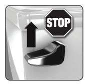
At the first sign of a clogged toilet, push handle upward as shown in the picture to the left.
