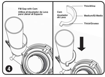
If gap appears around overflow tube, estimate width of space and use with thick, medium or thin section of Cam, as needed to fill gap.
