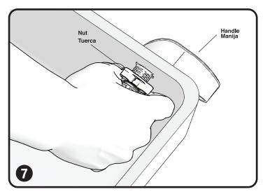
Tighten nut onto Handle.
