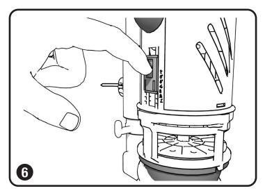
The blue adjustable slide controls how much water is used each flush. The higher it is raised, the less water is used. On most modern 1.6 or 1.28 GPF toilets, it can remain at the lowest settings. On older toilets, you may see some water savings from raising it.
