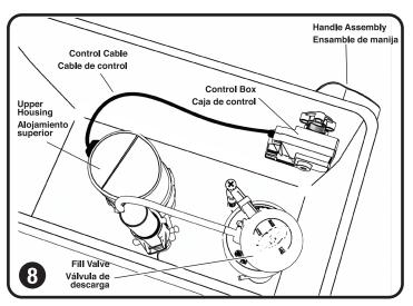
Position handle in standard operating position and attach gray control box to Handle Assembly. Audible click assures that Clip has secured Control Box to Handle, and unit will no longer pull apart without pushing the Blue Push Release. CONTROL BOX AND CONTROL CABLE MUST NOT TOUCH FILL VALVE OR INTERFERE WITH FILL VALVE'S OPERATION.
