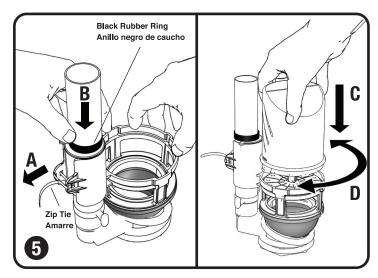
While applying downward pressure on the top of the base assembly, pull the zip tie (A) tight. B. Slide the black rubber ring onto the overflow tube until it just makes contact with the top of the base assembly bracket.
