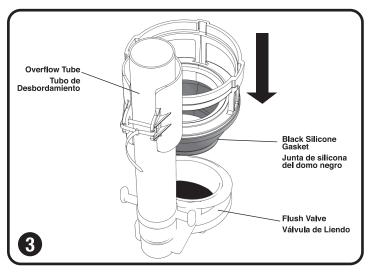
Slide Base down overflow tube, seating Black Silicone Gasket into flush valve
