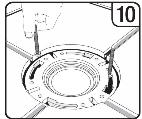
If old bolts are being re-used to set toilet, wipe clean with paper towel and re-install them in floor flange. If using new bolts, replace bolts in floor flange.
