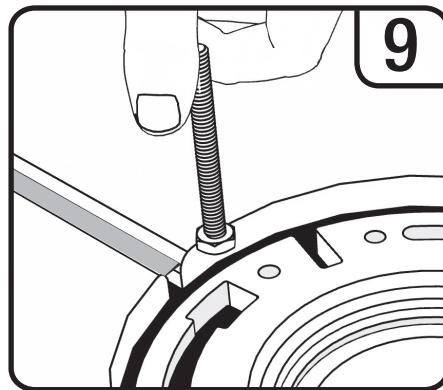
Remove bolts from floor flange and set aside. If floor flange is damaged, replace. Use putty knife to scrape off wax and residue from the floor flange. Wipe clean with paper towels. It does not need to be perfect.
