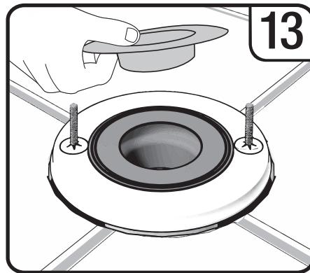
Place the HydroCap over the bolts and press down to seal. Once the HydroCap is pushed down onto the wax, use the star washers to secure the bolts. To lock them in, pull up on the bolt as you press down on star washer. The star washers snugly hold the bolts upright for easy installation. **Warning: Please make sure to remove Debris Cover before resetting toilet.**
