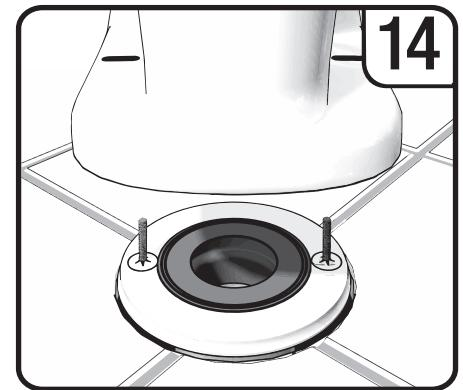
Line up the bolts through the holes in base of toilet bowl and reset the toilet. Use body weight to compress wax. CAREFULLY tighten bolts down evenly, alternating sides until snug. If the bolts were replaced, use a hack saw to cut off excess bolt just above the nut. Replace the decorative caps. Reconnect water supply line (we recommend replacing old, stiff supply lines with a new, flexible supply line). Turn on water and check supply line for leaks. Your toilet is ready for use.
