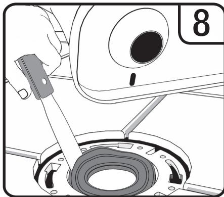
CAREFULLY lay the toilet on its side or tilt toilet and wipe off old, waxy residue from underside of toilet base with paper towels.
