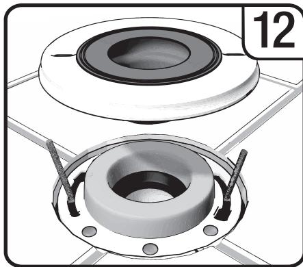
Place HydroCap Sure Seat Wax Ring Cap over the bolts and check height.
