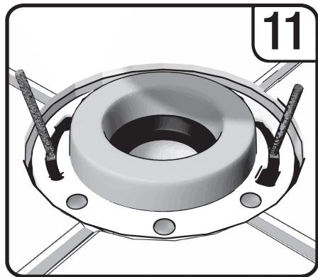
Set wax ring onto floor flange. **DO NOT USE PLUMBER'S PUTTY.**
