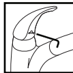
Unscrew set screw with Hex. (The set screw is directly underneath the handle.)
